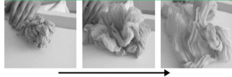
Shape memory textile (Grado zero innovation, 2021)
